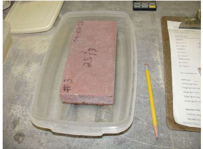
Figure 3—Specimen Undergoing the Water Uptake Test Method
