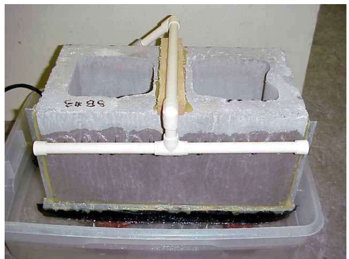
Figure 2—Specimen Undergoing the Spray Bar Test Method
