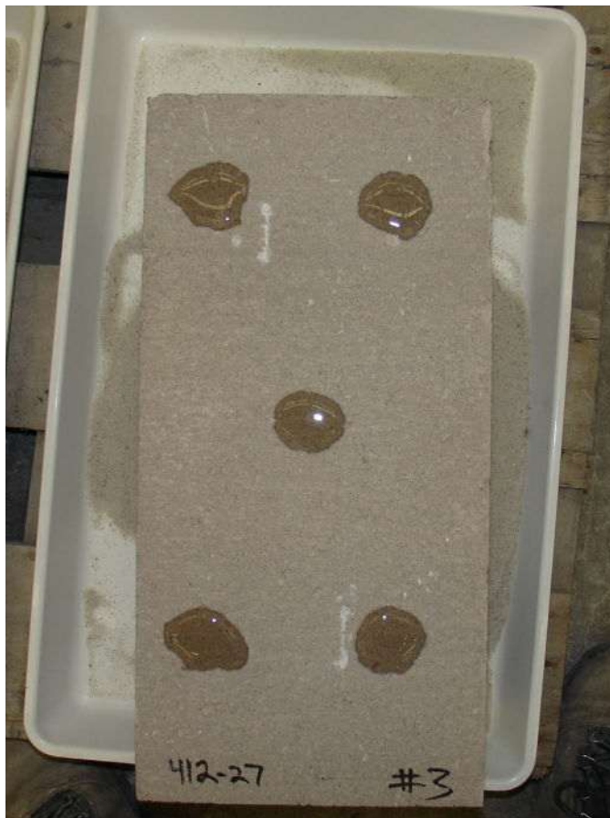
Figure 1—Specimen Undergoing the Water Droplet Test Method
